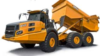
As coal is lighter and less abrasive than typical overburden, the steel plate used in coal bodies is not as thick as standard ADT load bodies. As a result it cannot be used to haul more aggressive materials. Tailgates are supplied with coal bodies.
